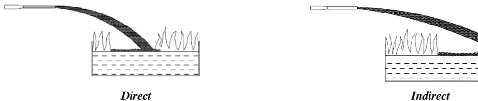
Application method- and technique is determined by the choice of equipment and type of fire to be extinguished. All units making up the total extinguishing system must be designed and dimensioned so that it is adapted, or suitable, to the potential scenario one would be confronted.
